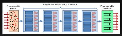
P4 pipeline architecture, showing the path every packet traverses through a P4-capable device <sup>1</sup>
